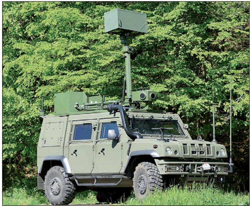
■ SRTP: a passive reconnaissance system designed for detection, survey and identification of radar and radio signal sources. Its core represents the radio signal analyzer that allows to perform pulse and continuous signal analyzes that are fed to its inputs at the intermediate frequency level with an adjustable bandwidth between 1 MHz and 200 MHz in the frequency range from 0 to 500 MHz.
