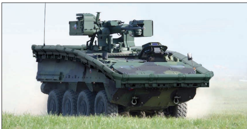
■ PAO: is the advanced active ballistic protection for the current and newly introduced military equipment of the Czech Armed Forces against attacks by RPG and PTRS. The System is designed to protect the entire vehicle, including the ceiling, and is also suitable for the light and moderately armored vehicles. The system consists of detection and tracking subsystem, control subsystem, and countermeasures with an initiating subsystem.
