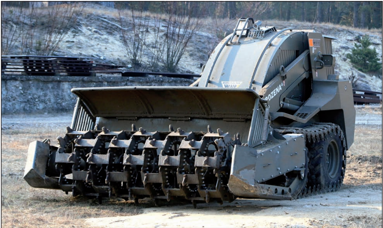
■ The Božena 4+ mine clearance system has a more powerful engine, a wider chassis, and a more efficient rotary mine
