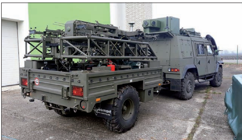
■ RAPAMEP: is a passive reconnaissance system designed for detection, survey and identification of radar signal sources. The RAPAMEP is a direction finding ELINT system for fast detection and identification of radar signals in the frequency range from 30 MHz to 1600 MHz.
