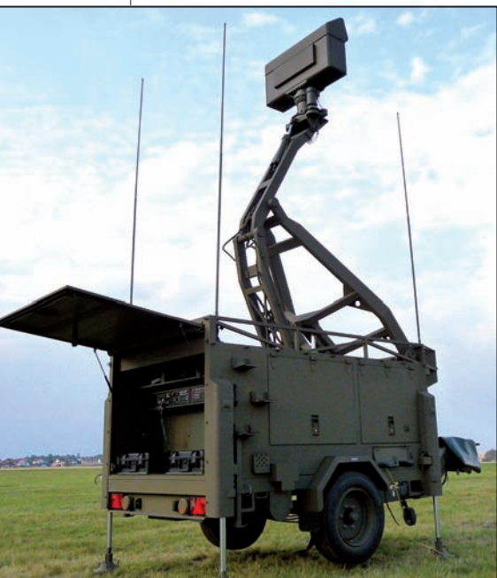
■ In recent years, The RETIA has delivered ReVISOR radars to the Czech Army.
