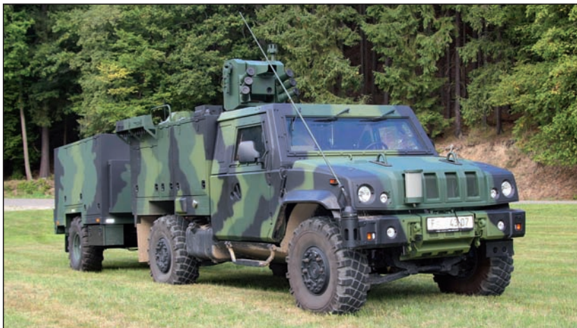
■ S-LOV-CBRN: a set consisting of light armoured reconnaissance vehicle S-LOV-CBRN and trailer P-LOV-CBRN. The set is intended to conduct (a) mobile CBRN reconnaissance, (b) long-term CBRN monitoring on observation point and (c) automated remote CBRN monitoring to protect the critical elements of combat formation.
