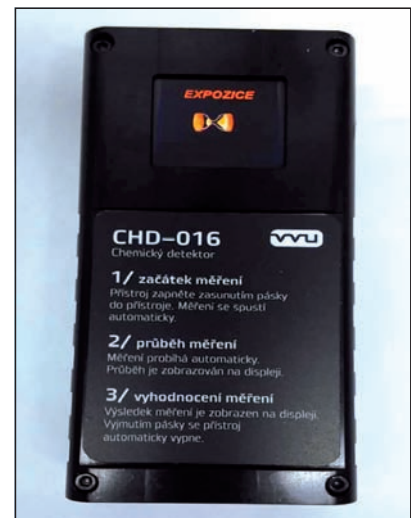
■ CHD-016: highly sensitive detector of nerve CWA. The detector is intended for sensitive detection of agents inhibiting cholinesterase in living organisms. It mainly concerns nerve CWA of „G“ type (i.e. SARIN, SOMAN, TABUN etc.) and „V“ type (i.e. VX), which represent high risk resulting from their toxicity as well as from their physical and chemical properties. Also, it is possible to detect the TIC inhibiting cholinesterase, like selected pesticides etc.
